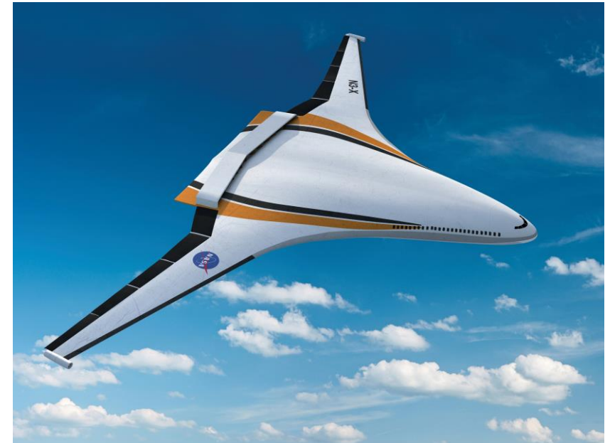
NASA N3-X Eco friendly electric airplane (wing-body with turbo-electric propulsion)
